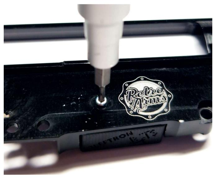
Lube the bottom part of the spring and trigger end with a small amount of grease. It will make smooth trigger pull.
